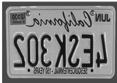
Reversed from left to right, as viewed using a Star Diagonal on a refractor.
